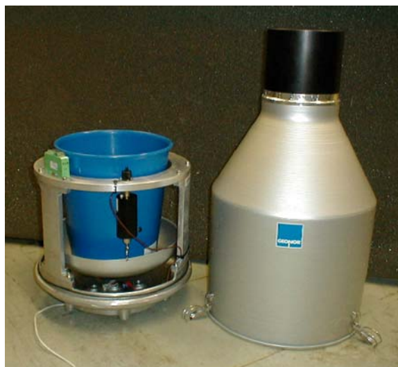
Figure 1. Geonor precipitation gauge, showing housing, bucket, and transducer/wire.
