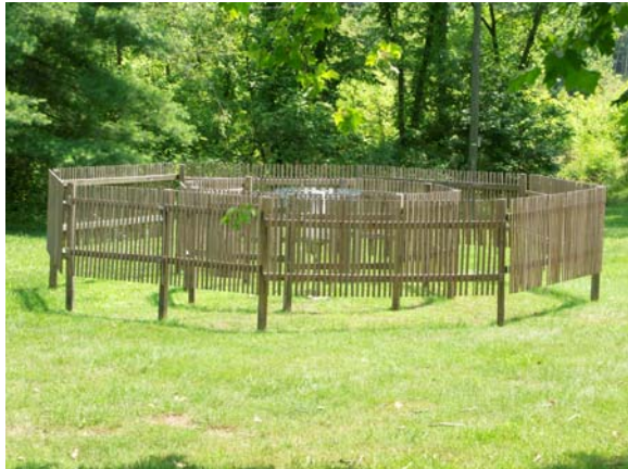
Figure 2. Double fence (DFIR) surrounding the Geonor precipitation gauge.
