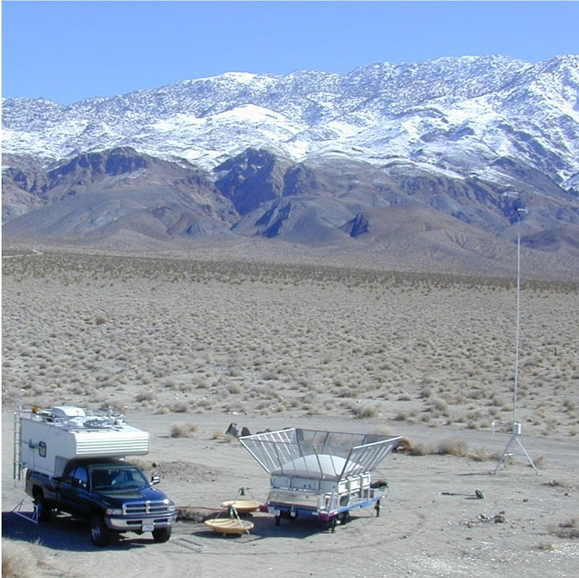
*Figure 1: Mobile Integrated Sounding System during the Sierra Rotors Project. The truck and camper are at left (with MotoSat communications antenna and net radiation sensors on the camper roof), the trailer with wind profiler antenna and clutter screen at center (small dishes between are the RASS acoustic source/reflectors), and the 10-m surface tower is at right. The Inyo Mountains east of Owens Valley are in the background.*
