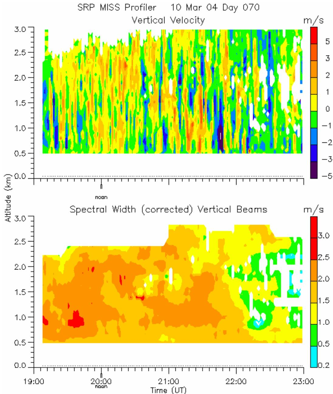
Figure 6: Vertical wind speed (top, negative values downward) and Doppler spectral width (bottom) measured with the MISS vertically pointing beam during the first 4 hours of IOP#2.
