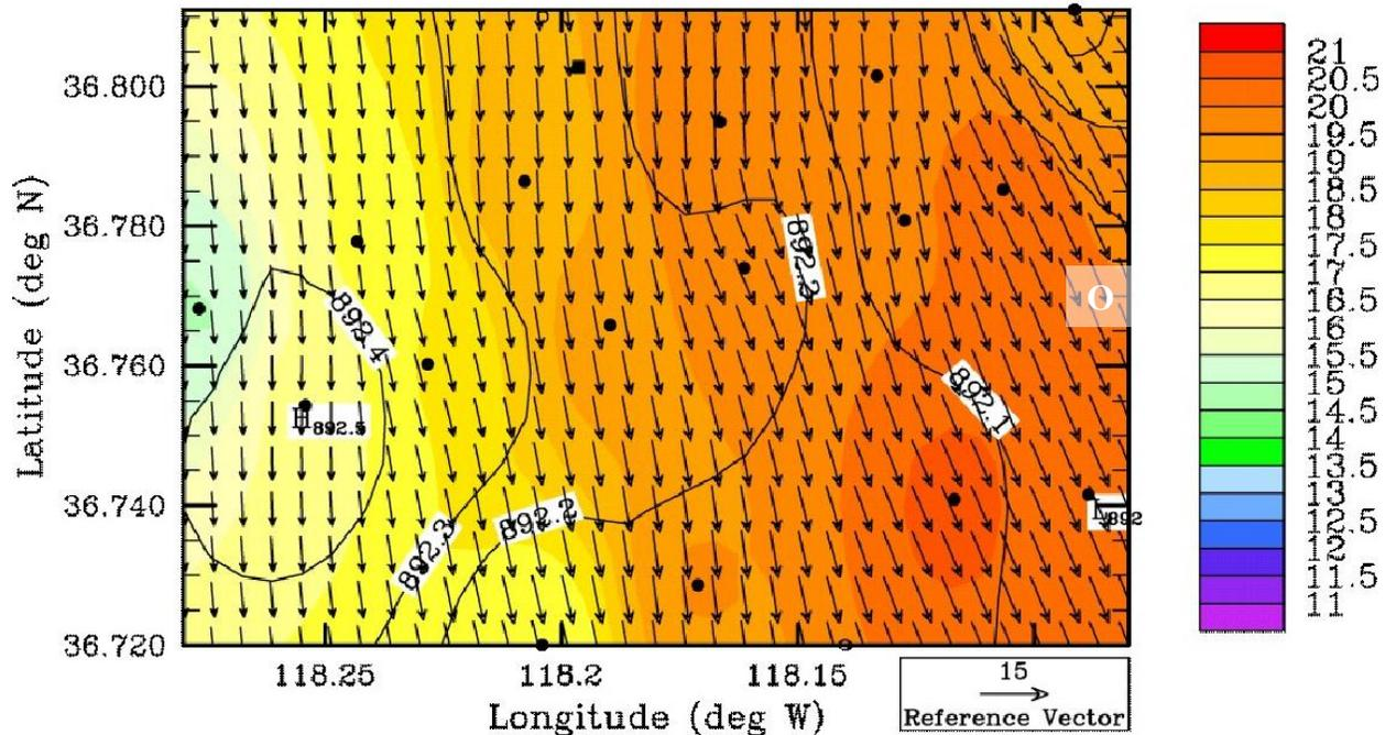
Figure 4: Vector winds ( $\text{m s}^{-1}$ ), temperature ( $^{\circ}\text{C}$ , color), and pressure corrected for the valley slope (hPa, contours) at 19 UTC on Mar. 10. There is a well established down-valley (NNW) flow. The MISS site is indicated by the white circle (right side), and black dots are the sites of the DRI surface (automatic weather station) network.
