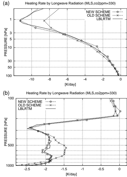
Fig. 4. Heating rate by longwave radiation for midlatitude summer profile. (a) Above 100 hPa, (b) below 100 hPa.
