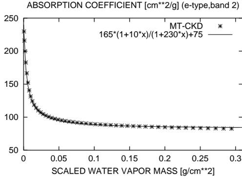
Fig. 2. Absorption coefficient for e-type absorption in the 2nd band. Results by MT-CKD model (\*) and by fitting (solid line) are shown. Abscissa represents scaled water vapor mass divided by 1013 hPa.
