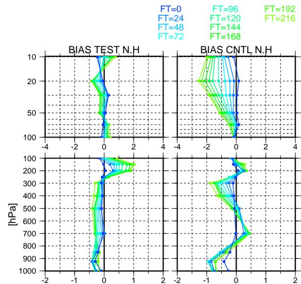
Fig. 6. Vertical profile of temperature bias against sonde observations at the Northern hemisphere ( $20^\circ N-90^\circ N$ ) in August 2004. Left panel is by the new scheme, right is by the old scheme. Each line represents bias for forecast time from FT00 to FT216 hours.
