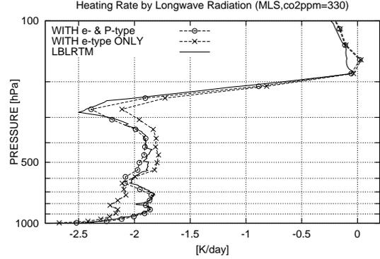
Fig. 3. Heating rate by longwave radiation for midlatitude summer profile. Results by calculation with ( $\circ$ ) and without ( $\times$ ) P-type absorption and line-by-line method (solid line) are shown.
