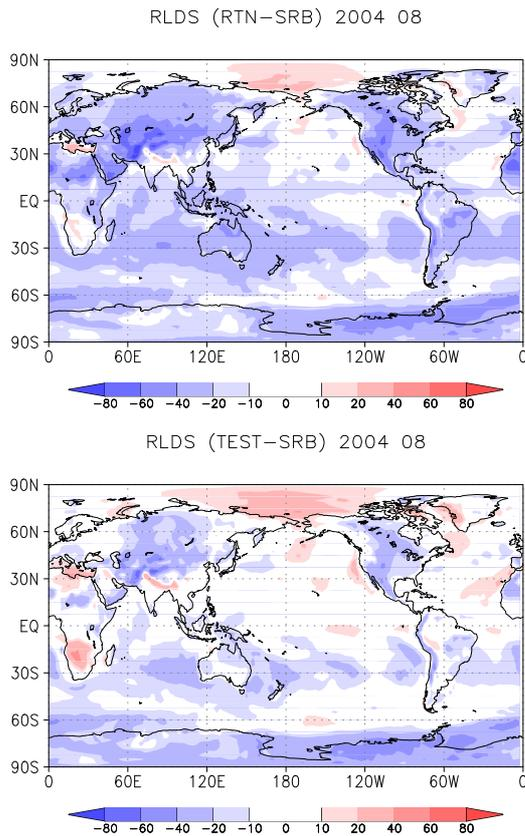
Fig. 5. Error in downward longwave radiative flux at the surface against SRB. Unit is  $W/m^2$ . Upper panel is for old scheme, lower is for new scheme.
