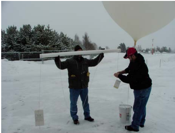
Figure 3. Simultaneous Radiosonde Launch at Caribou, Maine.
