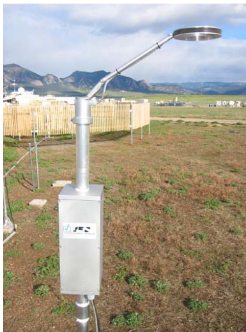
Figure 1 - The Hotplate snow gauge deployed at the NCAR Marshall Field Site just south of Boulder, CO.
