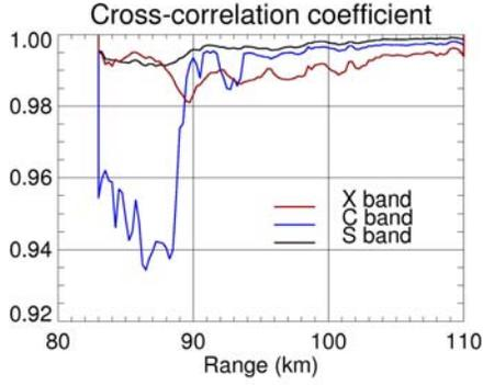
Fig. 8 Simulated radial profiles of  $\rho_{hv}$  at S, C, and X bands derived from the KOUN data at  $Az = 114^\circ$  (Fig. 5).
