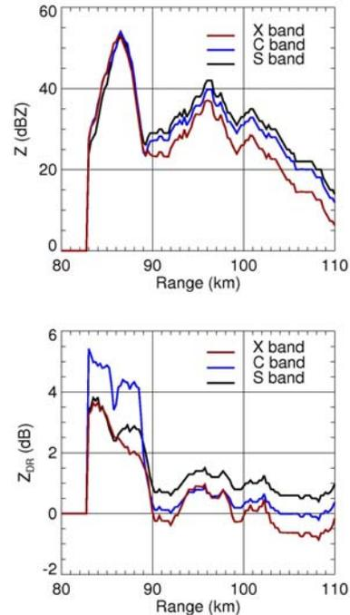
Fig. 6 Simulated radial profiles of  $Z$  and  $Z_{DR}$  at S,C, and X bands retrieved from the KOUN data at  $Az = 114^\circ$  (Fig. 5).
