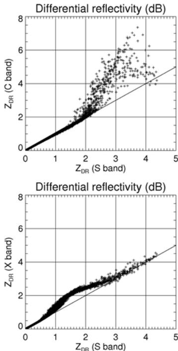
Fig. 2.  $Z_{DR}$  at C and X band versus  $Z_{DR}$  at S band as derived from disdrometer data.
