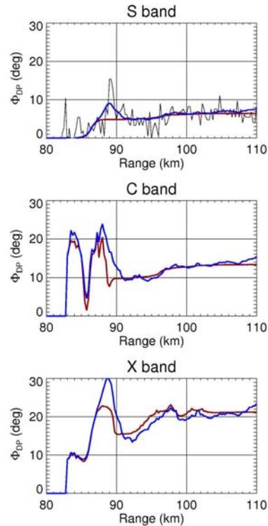
Fig. 7 Simulated radial profiles of  $\Phi_{DP}$  at S, C, and X bands retrieved from the KOUN data at  $Az = 114^\circ$  (Fig. 5). Blue lines – nonuniform beam filling (NBF) is accounted for; red lines – NBF is not accounted for. Black line in the top panel depicts  $\Phi_{DP}$  measured by KOUN.
