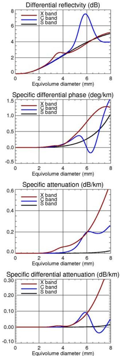
Fig. 1. Dependencies of  $Z_{DR}$ ,  $K_{DP}$ ,  $A_h$ , and  $A_{DP}$  on raindrop equivolume diameter at S, C, and X bands ( $T = 20^\circ\text{C}$ ).
