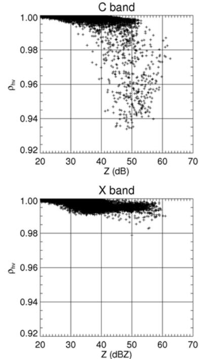
Fig. 3 Scatterplots of  $\rho_{hv}$  versus  $Z$  at C and X bands as derived from disdrometer data.
