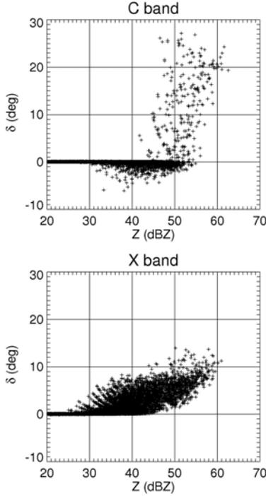
Fig. 4 Scatterplots of backscatter differential phase  $\delta$  versus  $Z$  at C and X bands as derived from disdrometer data
