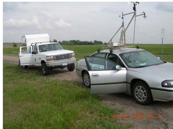
FIG. 1 – A photograph of the UMass W-band radar (left) and a mobile mesonet probe (right) shortly before dryline transects on 7 May 2005
