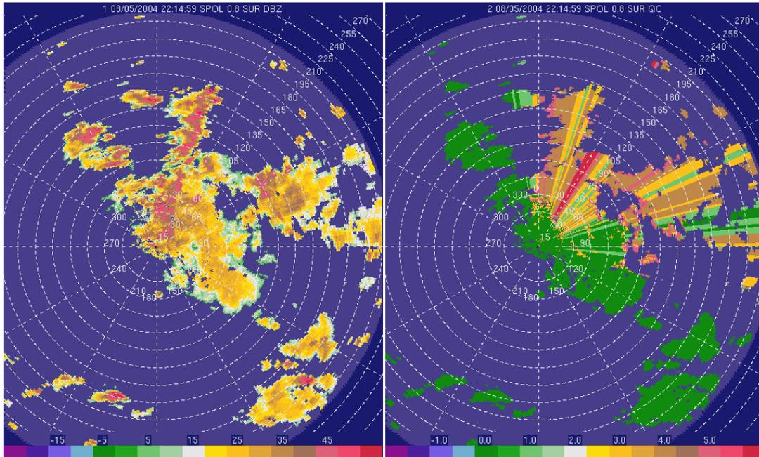
**Figure 3.** PPIs of reflectivity (left) and QC flags (right) for merged S-Pol data, using 3 elevation angles to correct blockage in the northeastern sector. In the QC field, 0 means unblocked 0.8°; 1 is blockage-corrected 0.8°; 2 is uncorrected 0.8° in a blocked region, but with no 1.3° or 1.8° echo available above the gate; 3 is unblocked 1.3°, 4 is blockage-corrected 1.3°, 5 is unblocked 1.8°, 6 is blockage-corrected 1.8°.
