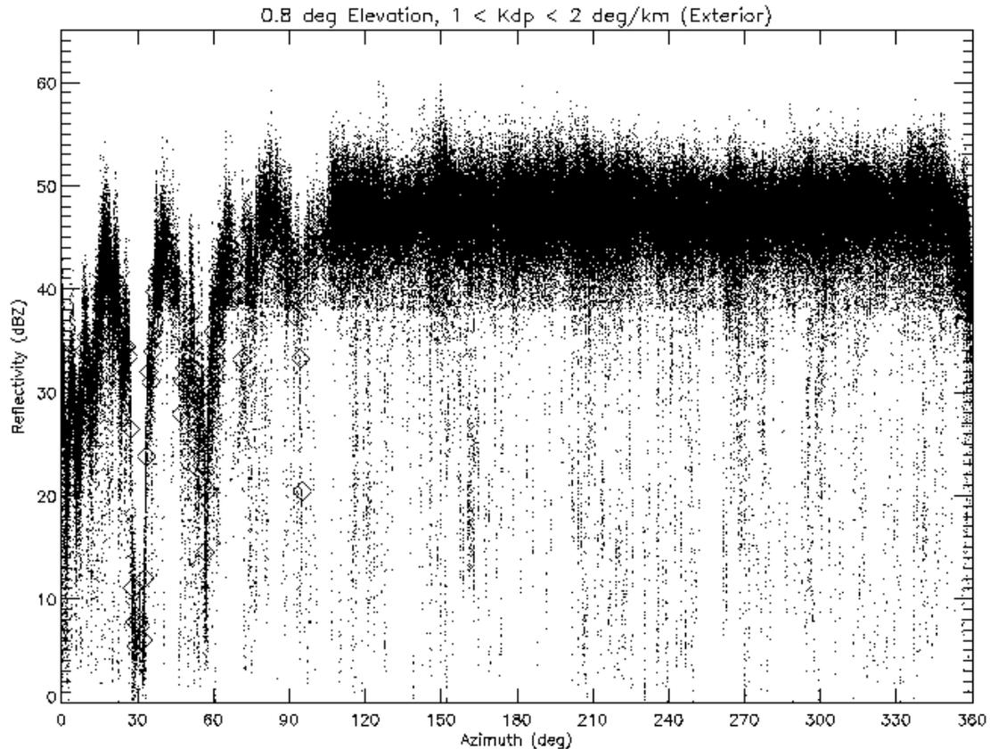
**Figure 2.** Reflectivity of S-Pol gates (dots) with  $K_{dp}$  between 1 and 2  $^{\circ} \text{ km}^{-1}$ , as a function of azimuth, for 0.8 $^{\circ}$  elevation angle. Data are Version 2 prototype S-Pol data from 8/2-8/9/2004 and include a filter on points with  $Z_h < 38$  dBZ and  $\Phi_{dp} < 15^{\circ}$ . Diamonds are median reflectivities at each azimuth.
