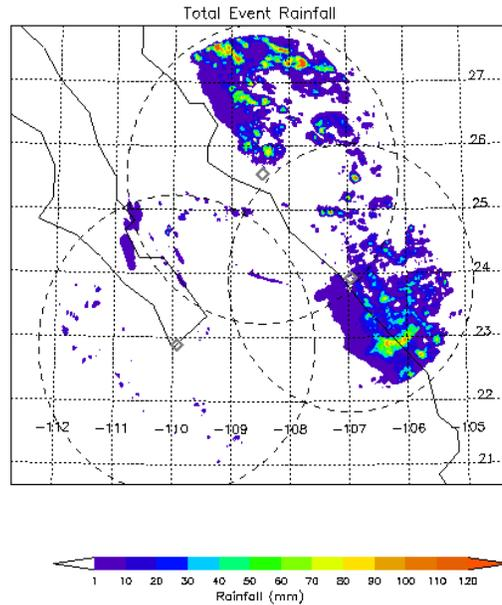
**Figure 1.** Example rainfall product demonstrating the NAME radar network geometry. Cabo is the westernmost radar, Guasave the northernmost, and S-Pol the easternmost (gray diamonds). Maximum range rings (dashed curves) and lat/lon grid also shown. Product is total rainfall for 17 July 2004.
