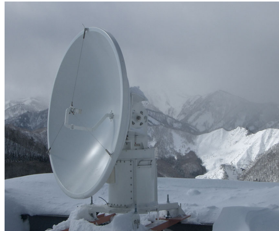
Fig. 1 The portable X-band radar on the rooftop of the building during the orographic snow cloud modification field program.
