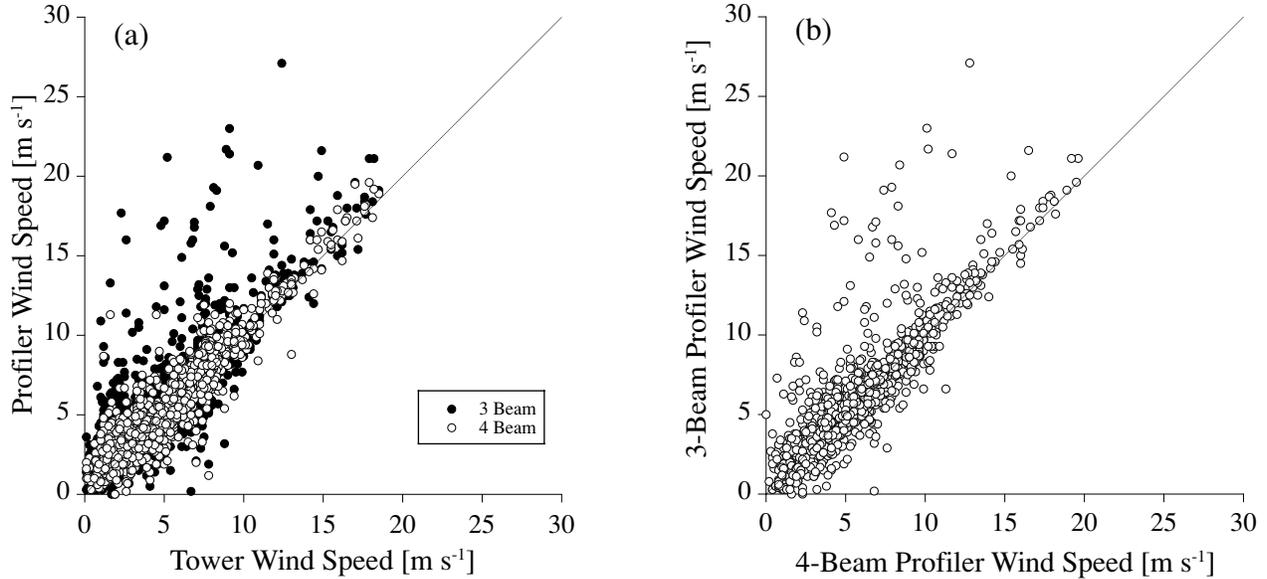
Figure 2. Scatter plots of the wind profiler versus the tower speed (a) and of the three-beam system versus the four-beam system (b) measured at about 200 m for clear-air. The data derived from the three-beam (four-beam) system is plotted as closed (open) circles in (a). The data were averaged over thirty minutes. The lines are 1:1.
