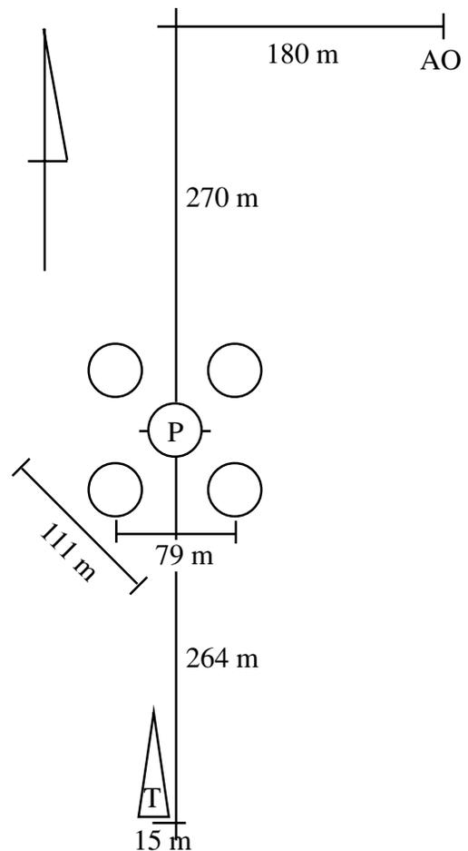
Fig. 1. Schematic layout of the relative locations of the meteorological tower (T), the 1.3-GHz profiler (P), and Aerological Observatory (AO). The footprint of the 10° vertical profiler beam at 200 m is shown to scale as a circle around the P; circular approximations of the footprint and location of the oblique beams at 200 m are indicated by circles to the NE, SE, SW, and NW of the vertical beam.
