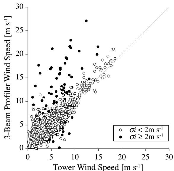
Figure 3. Scatter plots of the three-beam method profiler wind speed versus the tower wind speed measured at about 200 m, for conditions classified as clear-air using the vertical beam of the profiler. Data from half-hours with inter-beam standard deviation ( $\sigma_i$ ) greater than or equal to (less than)  $2 \text{ m s}^{-1}$ , i.e. during patchy rain (no rain in any beam) are plotted as closed (open) circles. The thick line is 1:1.
