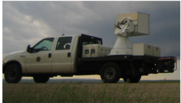
Fig. 1. Dual-polarization spaced-antenna (rectangular box) mounted on the mobile X-Pol radar positioner.
