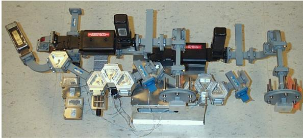
Figure 9. Ku-band front-end assembly.
