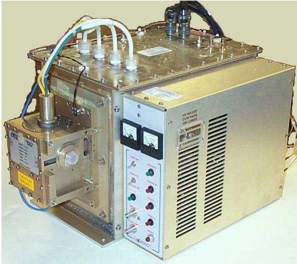
Figure 14. Conduction cooled W-band EIK VKB2461 (CPI) and the pulse modulator MG-1359 (Pulse Systems).
