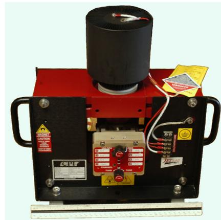
Figure 4. Ku-band EIK transmitter (CPI).
