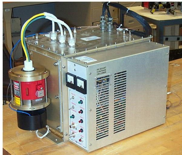
Figure 12. EIK VKQ2471 (CPI) and the pulse modulator MG1369 (Pulse Systems).
