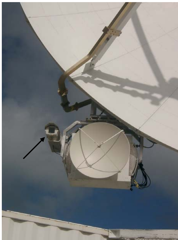
Figure 1. Photo showing network camera enclosure mounted to side of Ka-band radar; Ka radar is mounted to large S-band dish. Arrow indicates camera; Ka dish is 0.7 m diameter (28 inches). Photo courtesy J. Hurst.
