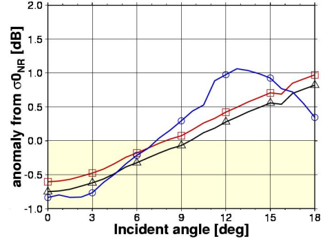
Fig. 3. \Delta\sigma_R^0 (triangle, black), \Delta\sigma_{ref}^0 (circle, blue), and \Delta\sigma_{fin}^0 (square, red) for different incident angles under weak rainfall less than 1mm/h over ocean.
