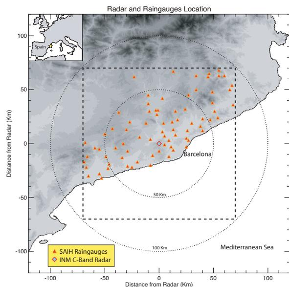
Figure 1. Map of the Barcelona area, showing the Barcelona C-band radar location (diamond), rain gauges (triangles) and range rings at 50 and 100 km from radar. Dashed square delimits the 140 x 140 km region that was used as study area.
