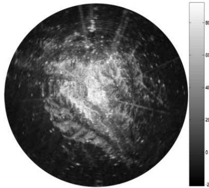
Figure 1: Average SNR, in dB. Map encompasses a 50 km radius around the KOUN research radar in Norman, Oklahoma.
