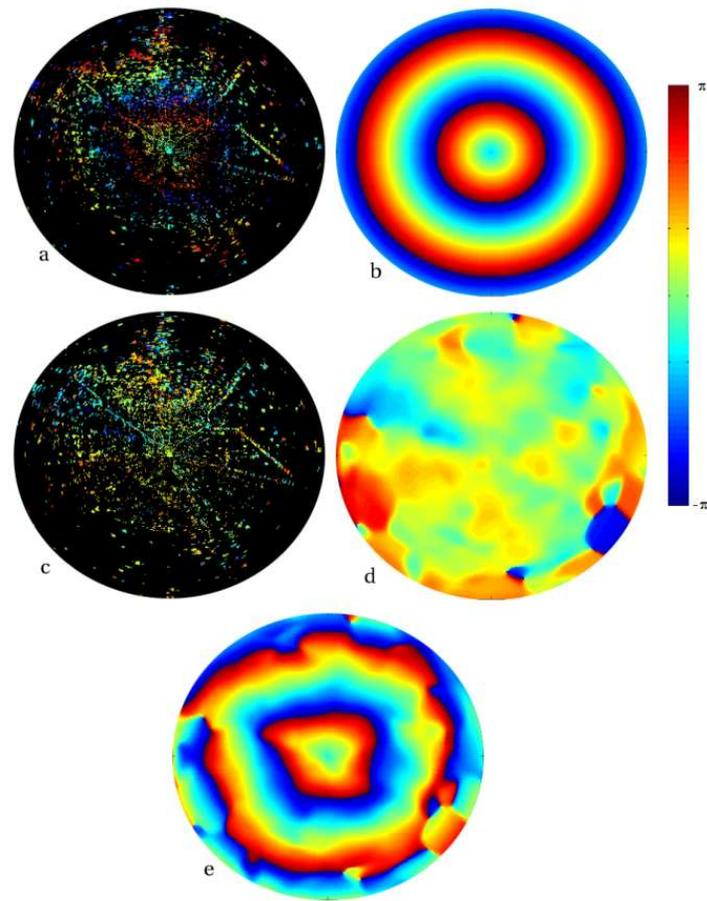
Figure 4: Phase difference estimation process: (a) phase difference between two times, (b) estimated average slope, (c) phase difference after removal of average slope, (d) smoothed phase difference, (e) phase difference field after average slope is returned.
