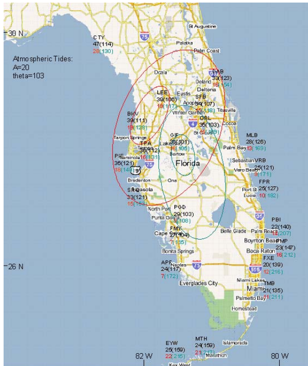
Figure 6: The diurnal component (black) and the mesoscale part (amplitude: red, phase: green) of the sea level pressure variations for stations in Florida. Amplitude is in unit Pascal. The red contours show the center of the amplitude. Phase angle is in unit Degree and in local solar time. The green contours show the center of the phase. The atmospheric tide in literature is taken as a reference.
