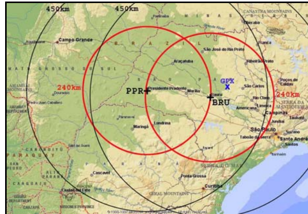
Figure 1. TroCCiBras Experiment Area, with IPMet's Radar Network (BRU = Bauru; PPR = Presidente Prudente), showing 240 and 450 km range rings. GPX = Base for TROCCINOX research aircraft.
