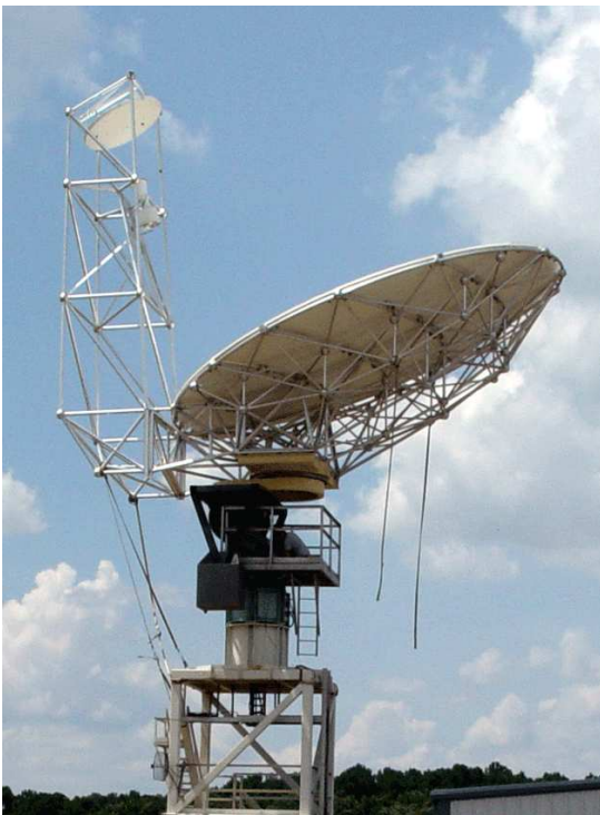
Figure 2: Offset-fed Gregorian Antenna
