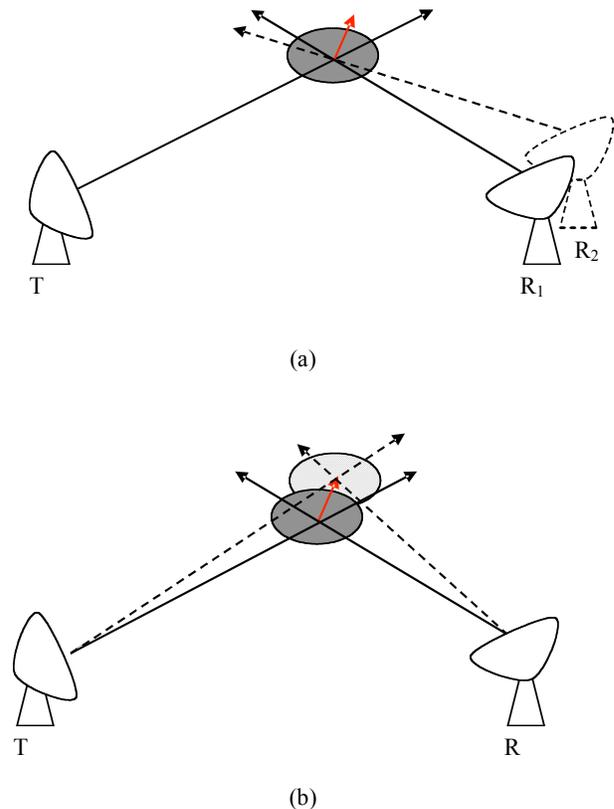
Figure 1: Configuration sketch of bistatic interferometry to measure transverse wind. (a) bistatic spaced antenna interferometry, (b) bistatic angular interferometry.
