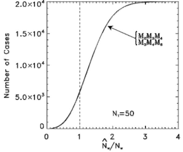
Fig. 8: Cumulative distribution of values of normalized gamma DSD concentration parameter  $\hat{N}_w$ , as estimated from the indicated sets of three sample moments. Abscissa indicates ratio of sample estimate to population value; vertical dashed line denotes population value. Population DSD: gamma,  $\mu = 2$ . Mean sample size: 50 drops.
