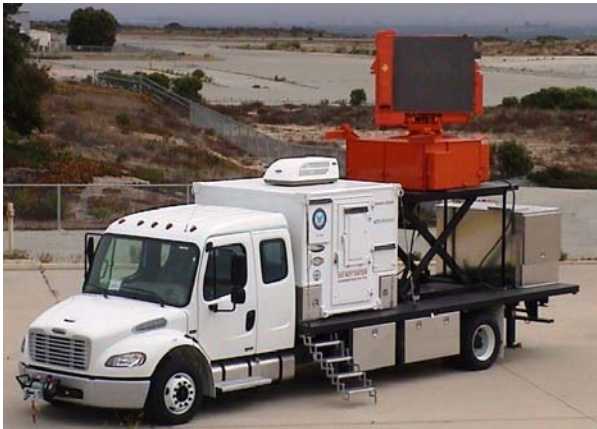
Figure 1 MWR-05XP installed on a heavy-duty truck. The 1.2 m phased array antenna provides electronic beam scanning in elevation and combines electronic back-scanning with mechanical scanning in azimuth.
