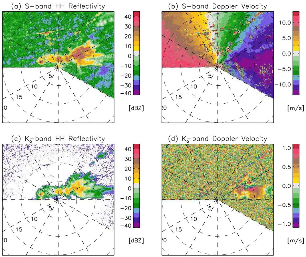
Figure 3: S- and  $K_a$ -band radar data collected during the RICO project at 14:48 on January 1, 2005. The elevation angle is 1.5 degrees. Concentric dashed rings indicate radial distance from the radar.
