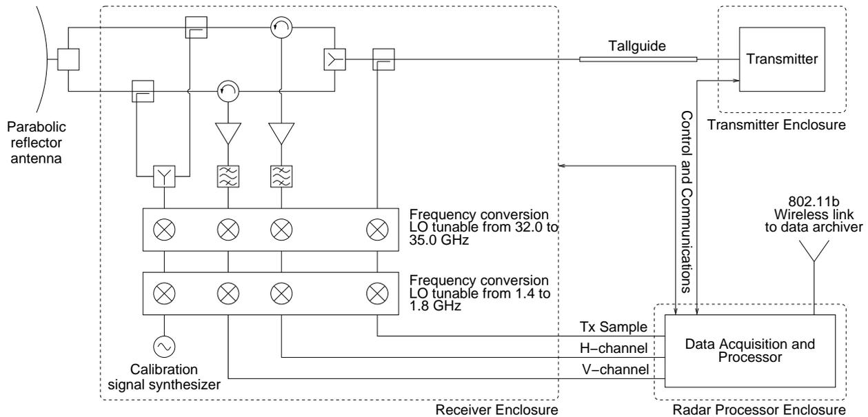
Figure 2:  $K_a$ -band block diagram. Dashed lines represent the three enclosures housing the  $K_a$ -band radar. The antenna is mounted to the receiver enclosure.
