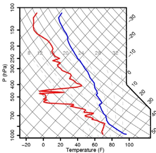
Figure 4 – SkewT-logP 1800 UTC 18 September 2002, Rondonia, Brazil. Temperature and dew point temperature are denoted by blue and red lines, respectively.
