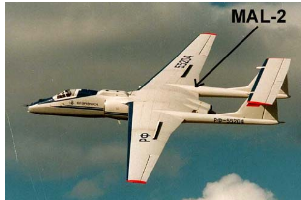
Figure 4. M55 Geophysica aircraft laboratory during TROCCINOX 2 (2005), indicating the position of the bay containing the MAL-2.
