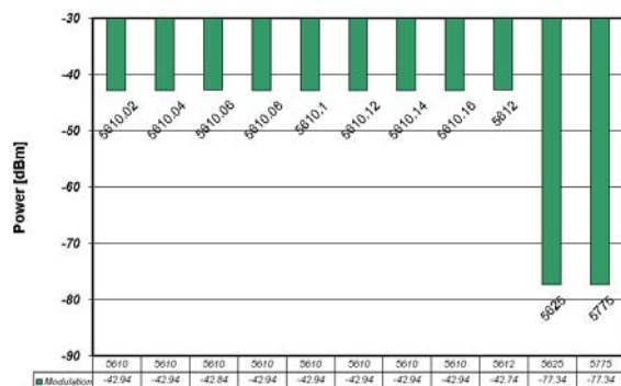
Figure 8: Frequency off-set variation. Variations of the order of a KHz have the same effect whereas shifts of 15 and 65 MHz in the RLAN carrier frequency are not detectable by the weather radar.
