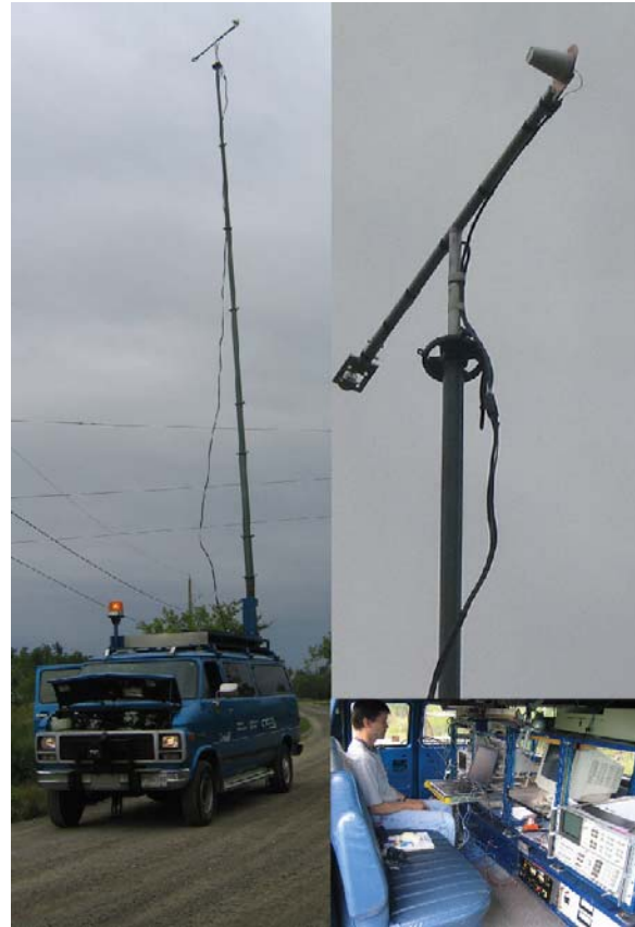
Figure 3: Experimental setup for the external tests, showing the 16 m (maximum) extendable mast (left) with the DFS detector and the RLAN antenna (upper right) and the RLAN equipment located in the van (lower right).
