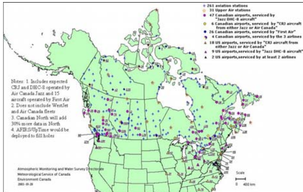
Figure 5.1 Projected weekly frequencies of aircraft ascent and descent soundings once Air Canada Jazz and First Air AMDAR Program components are fully developed and operational. A small aircraft icon represents an airport part of MSC's Aviation Surface Weather Network, a star a Canadian radiosonde site, and a colored circle an airport from which AMDAR soundings will be generated by Canadian aircraft.
