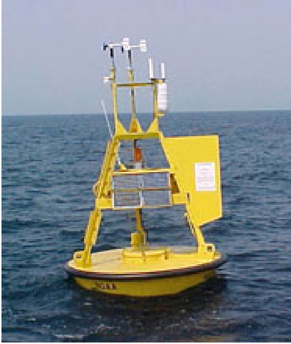
Figure 2. A typical moored NOAA buoy that provided the data for this study.
