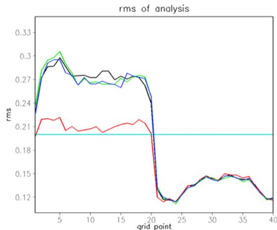
Fig.1. Five-year-average analysis RMS error for different methods (the straight line is the observation error standard deviation, the red line is RMS error from true ensemble variance method, the black line is the RMS error from ensemble spread method, the green line is the result of local  $P^a$  method, the blue line is the result of combined method ).
