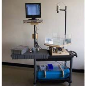
Portable rotating tank apparatus used to study the effects of rotation on geophysical fluid systems
