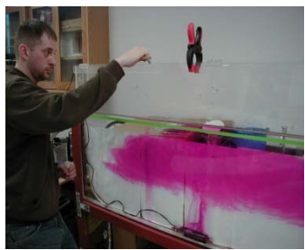
Millersville 2-D tank used to demonstrate convection, frontal boundaries, and fluid stability
