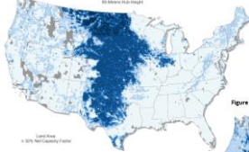
Figure 4-1. Land area achieving a minimum 30% net capacity factor by grid cell, based on 2005 technology
